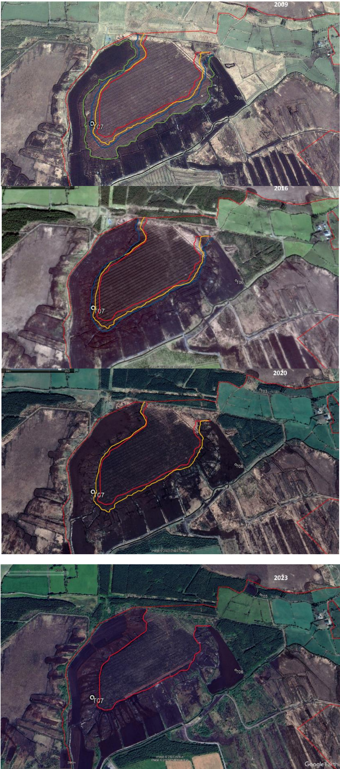
Figure 2-1: Peat cuts and harvesting at T07, showing the retreat of peat cuts from the turbine location (Google Earth, 2009-2023).
