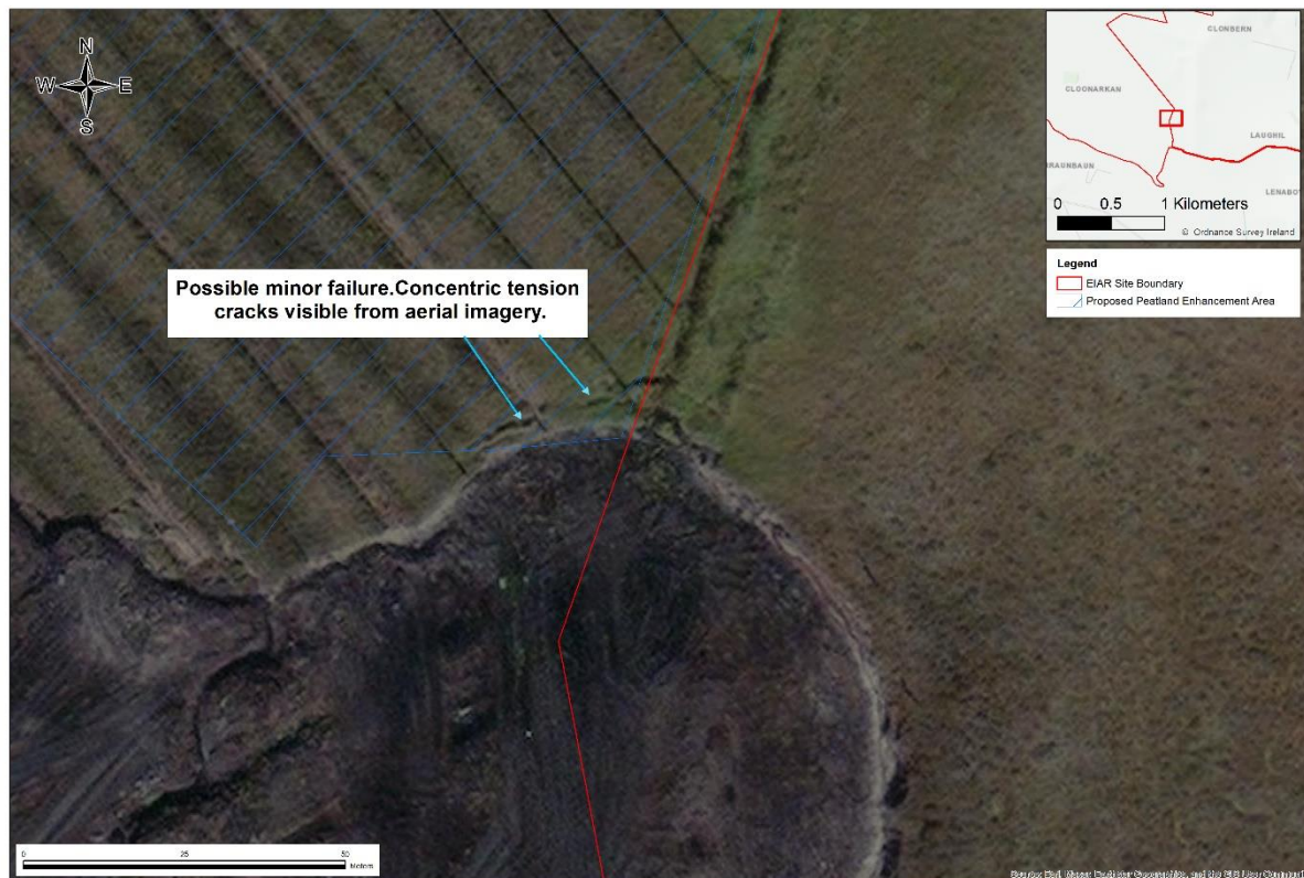
Figure 2-3: Possible minor failure at the southern edge of the area proposed for peatland enhancement as part of the Proposed Peatland Enhancement Area (ESRI World Imagery, 2020).
